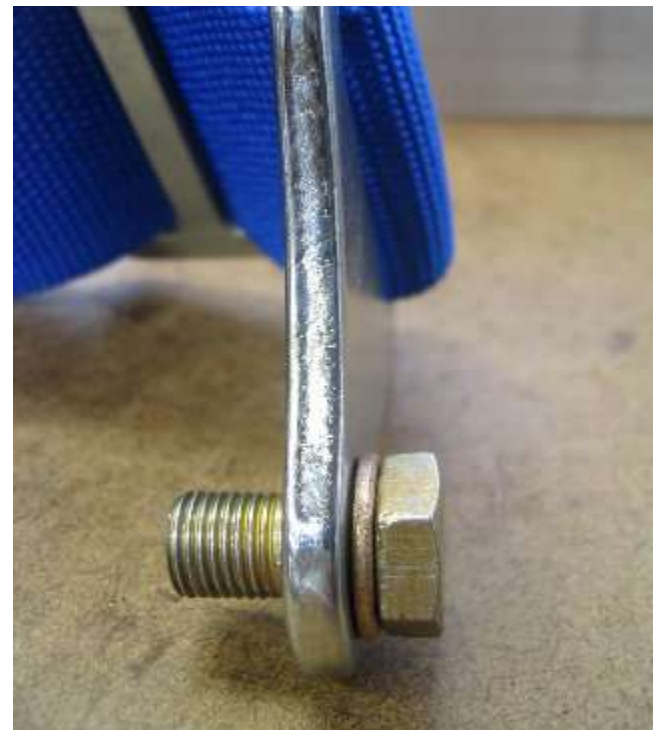
Photo 6 Harness Attach Plate, Flanged Bush, and AN6 Bolt
