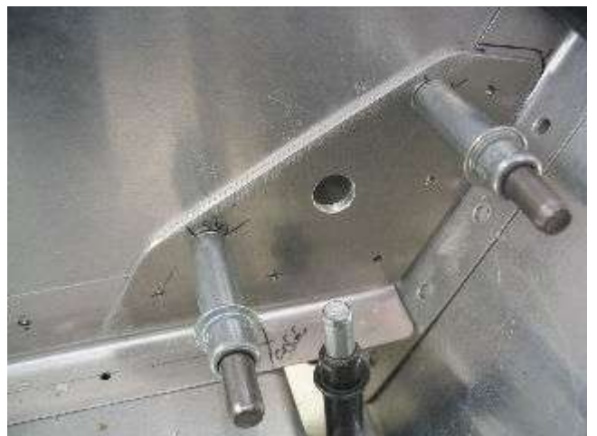
Photo 14 Installed Doubler and Shim for the inboard harness attachment
