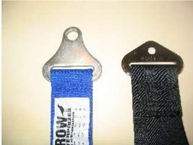
Photo 1 Comparison of the Harness Attachments Crow on Left, Zenith on Right
