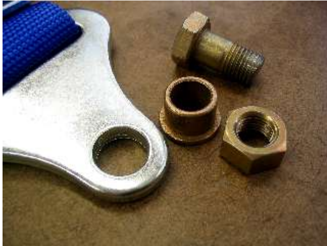
Photo 7 Harness Attachment Plate, Flanged Bush, and AN-6 Bolt
