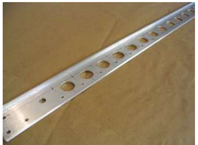
Photo 4 Lightening Holes in Aft Attach Point
