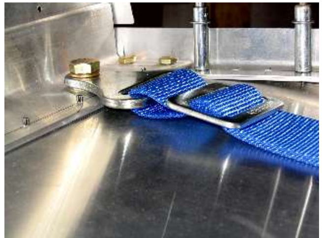
Photo 8 Aft Attach Point
