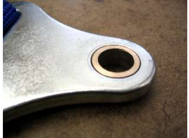
Photo 5 Harness Attach Plate and Flanged Bushing (Flange Hidden)
