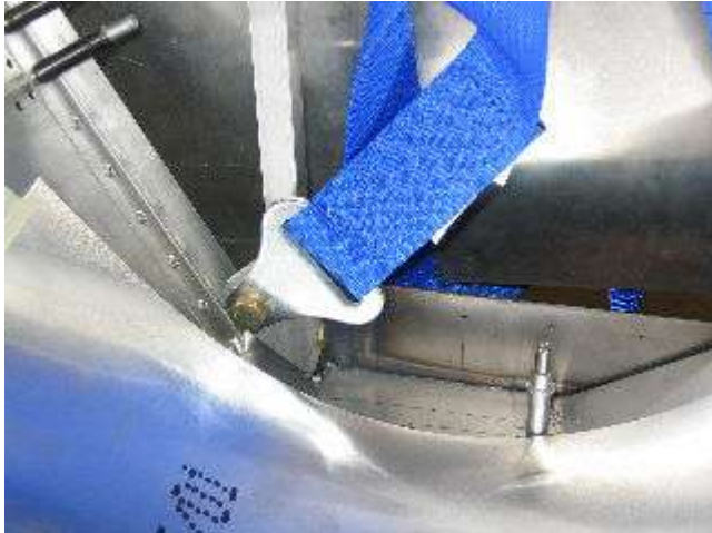
Photo 16 Detail of Outboard Attachment
