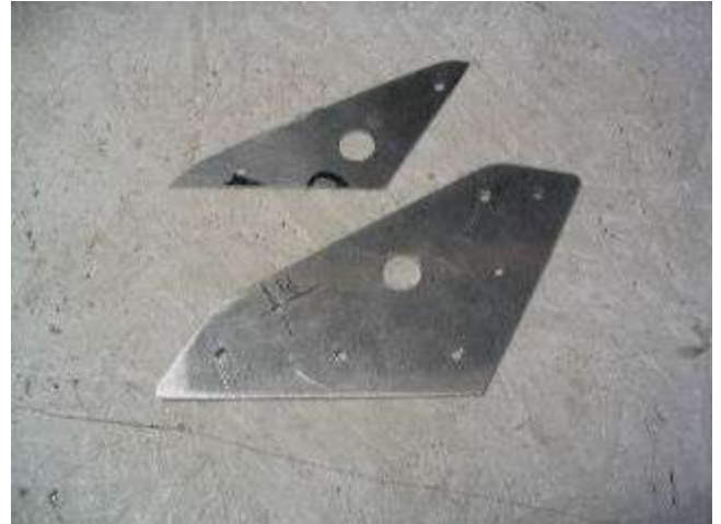
Photo 12 Shim and 6B18-3 Attachment Doubler Plate
