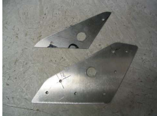
Photo 5 Shim and 6B18-3 Attachment Doubler Plate
